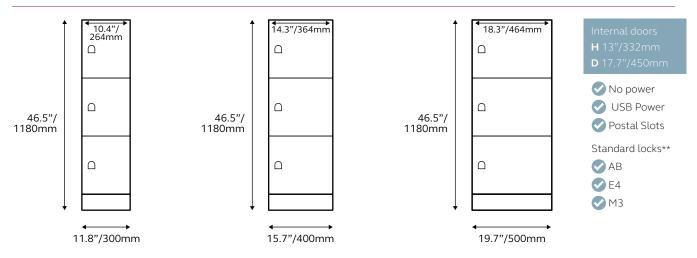
46.5"/1180mm high locker modules are not compatible with internal shelves
