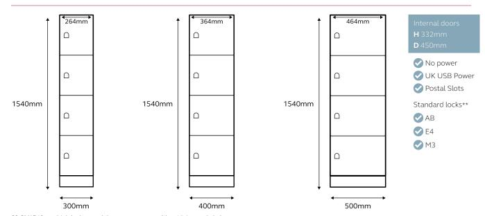
60.6"/1540mm high locker modules are not compatible with internal shelves.
